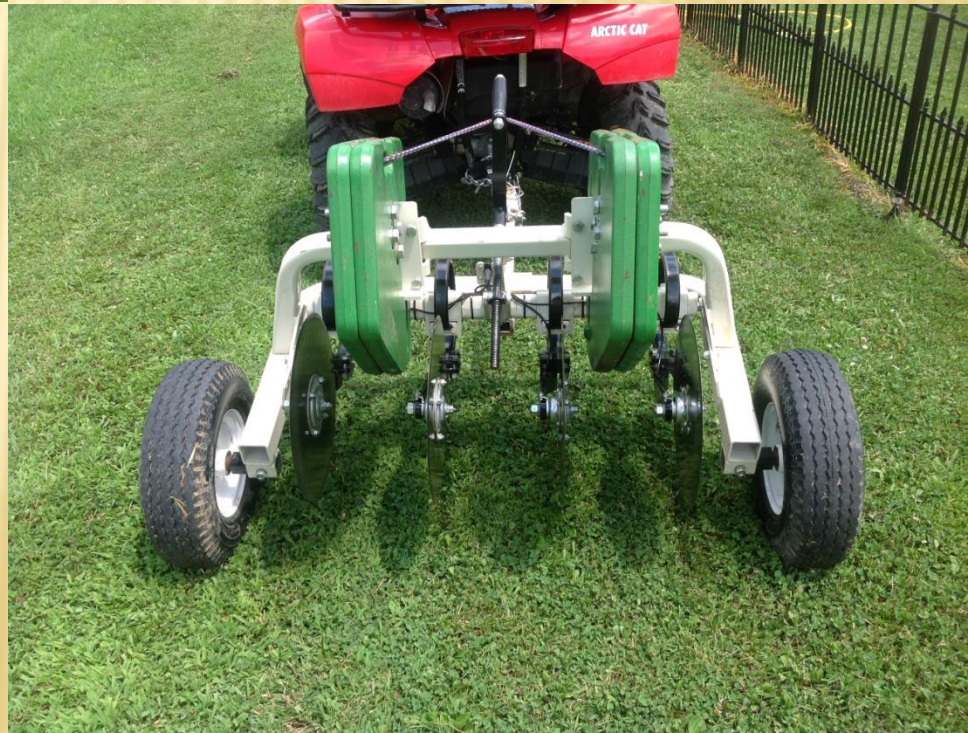
Rear View of the Veris Quad 1000 Soil Conductivity Sensor
