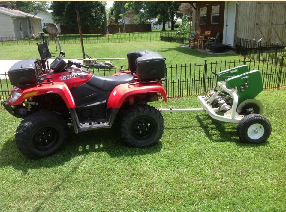
Side View of the Veris Quad 1000 Soil Conductivity Sensor
